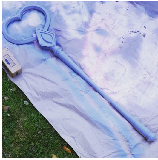
Staff is covered in Worbla, then sprayed with auto-filler and sanded for a smooth finish.
