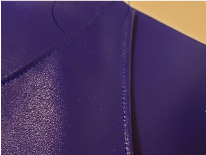
Top stitch all the seams by covering the pleather with wax paper and then tearing the paper away
